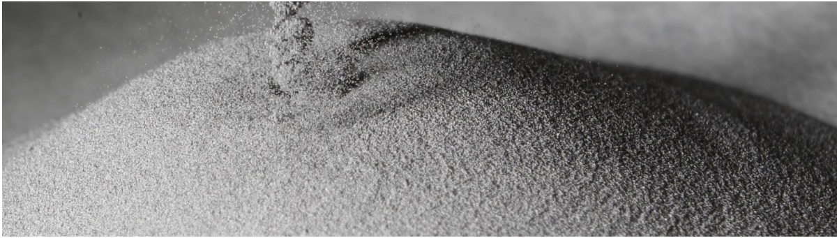
Image: PyroGenesis' titanium metal powder as produced by its NexGen™ plasma atomization system.
